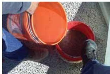
**Fig. 3:** Infiltration rate testing per ASTM C1701
