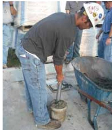
**Fig. 1:** To determine unit weight per ASTM C1688, concrete is consolidated using a Proctor hammer
