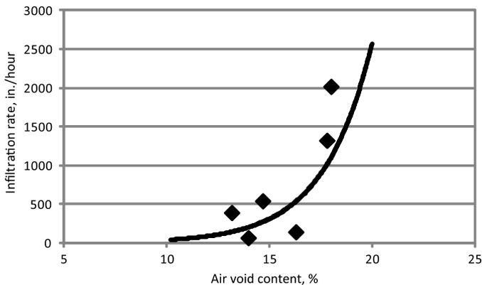
**Fig. 6:** Infiltration rate as a function of air void content. Note: 1 in. = 25.4 mm
