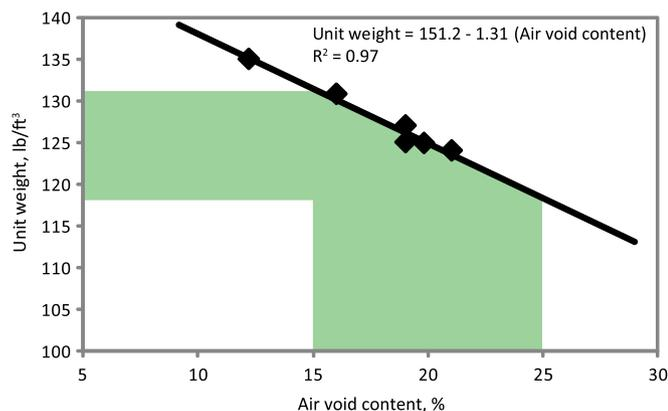
**Fig. 2:** Unit weight and air void content values for preliminary test panel concrete batches, measured per ASTM C1688. Note: 1 lb/ft<sup>3</sup> = 16 kg/m<sup>3</sup>
