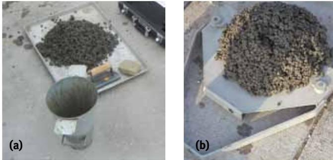
Fig. 4: Discharged concrete after inverted slump cone tests: (a) nonworkable mixture; and (b) workable mixture
